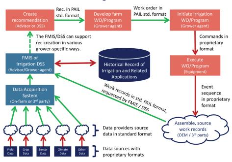
PAIL's vision for data flow in precision irrigation. Flow of data in a PAIL standard format is shown in green; flow of data in proprietary formats is shown in red.
