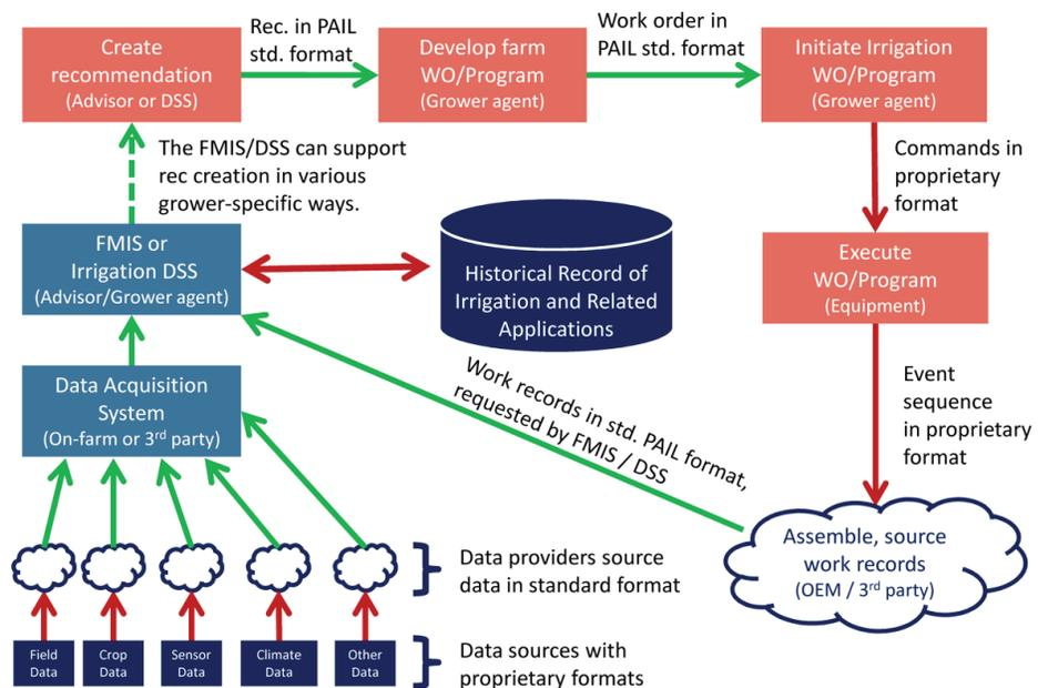
PAIL's vision for data flow in precision irrigation. Flow of data in a PAIL standard format is shown in green; flow of data in proprietary formats is shown in red.
